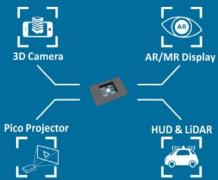
Our compact MEMS scanning mirror offers advantages for space and weight demanding applications such as AR/MR head mount display. A lightweight and compact near eye display solution can be achieved with fiber coupled RGB laser.
