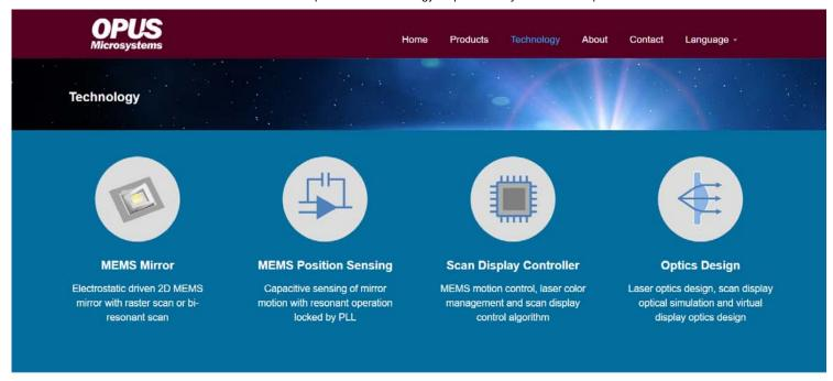
Our MEMS mirror device is packaged in the most compact format in the market. The mirror is monolithically integrated elestrostatic micro-actuator in single crystal silicon structure. No external components are needed unlike electromagnetic MEMS mirror which needs bulky magnets in mirror assembly. We have established MEMS manufacturing supply chain with world class partners for large volume production.
