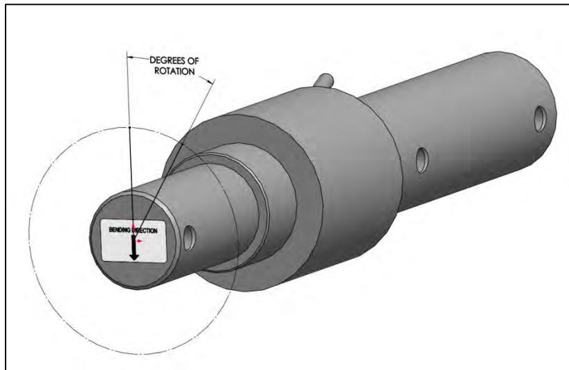
Underneath the cover is where all of the load cell circuitry is hidden away and protected from the elements. Without going into a lot of detail about how it all works, it's enough to say that the circuit is made of strain gages and other resistors wired into a Wheatstone bridge. The strain gages are positioned exactly on the top and bottom of the cell - that's how they are able to measure 100% of the load that is applied.
