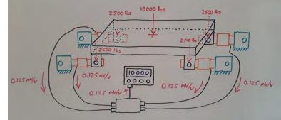
The load cells signals are also averaged in the junction box and sent to the indicator in the same manner:
