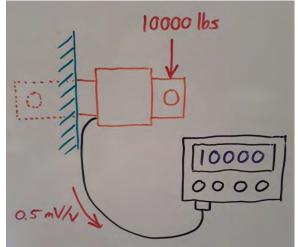
The output of a properly designed load cell is linear, which simply means that if you were to graph the output while changing the load, it would look like a straight line.
