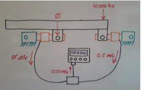
• The signals are averaged, and the resultant signal is sent to the indicator:
