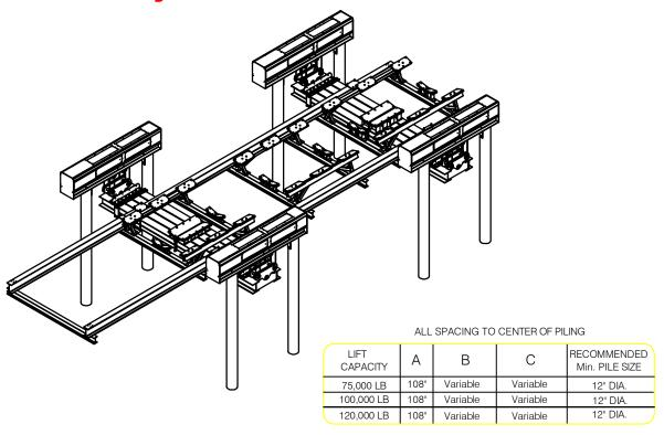
Dim B, C, and D are vessel/site dependent.
