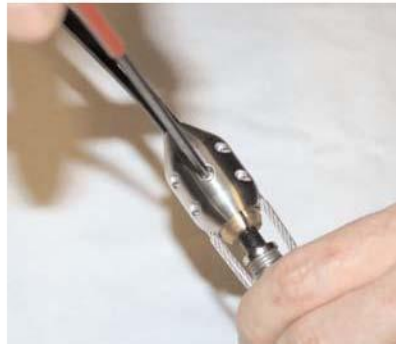
Tighten Cable connector with multi-tool
