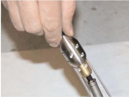
Slide Cable connector over Cable Reel fitting
