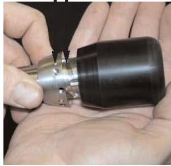
Aligning Dummy Plug with Cable Reel connector
