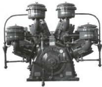
Compressor for Refrigerators
