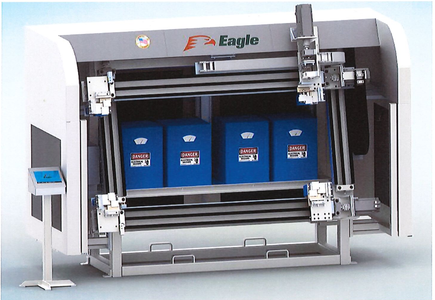
Cabinet Door Assembly Machine With Radio Frequency Gluing
