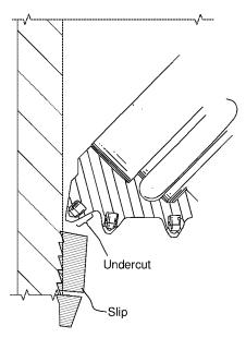
In the above figure, attempting to drill the hard slip will result in wear of the cone steel in the Undercut region before the insert is sufficiently exposed to drill through the slip.
