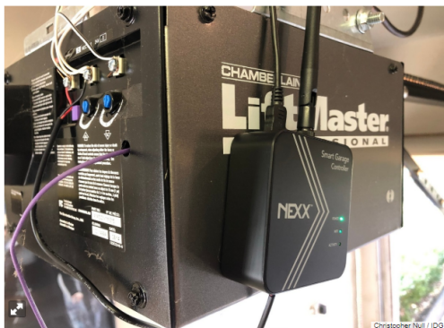
The Nexx NXG-200 must be attached to your garage door opener via wires, and space can be tight depending on your ceiling height.
