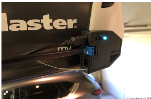
The Garadget fires a laser once a second at the door to determine whether it is open or closed. As with the product from NEXX, the Garadget must be hardwired to your opener.
