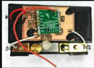
CCTV Shock Sensors
