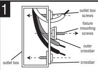
THREAD fixture mounting screws (provided) into outer cross
