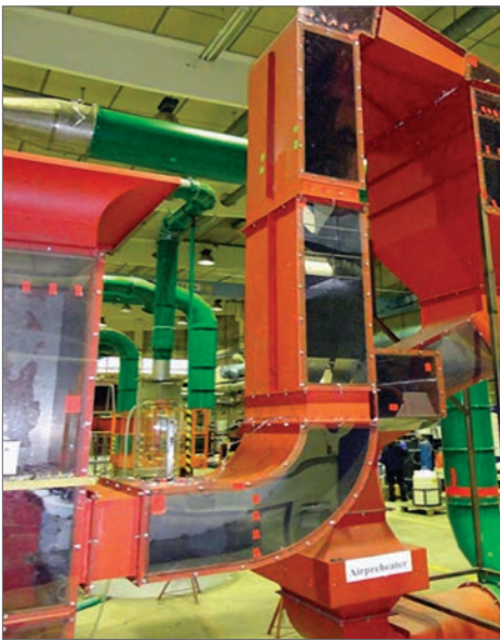
IsoSwirl™ prototype mixer undergoing performance testing at GE's research facility in Växjö, Sweden, one of the largest ECS research and development laboratories in the world.
