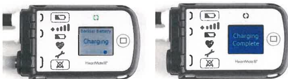
Figure 2.35 System Controller Charging or Charging Complete
