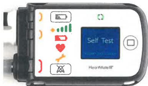
Figure 2.17 User Interface During System Controller Self Test
