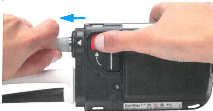
Figure 2.54 Grasp the Metal End and Remove the Driveline
