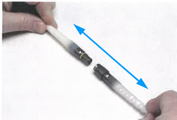
Figure 2.57 Pull the Connectors Apart
