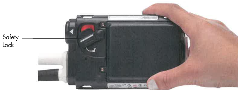
Figure 2.9 Move the Safety Lock to the Unlocked Position
