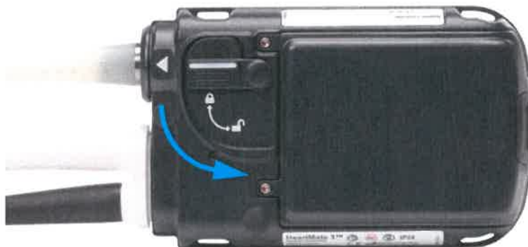
Figure 2.42 Unlock the Safety Lock
