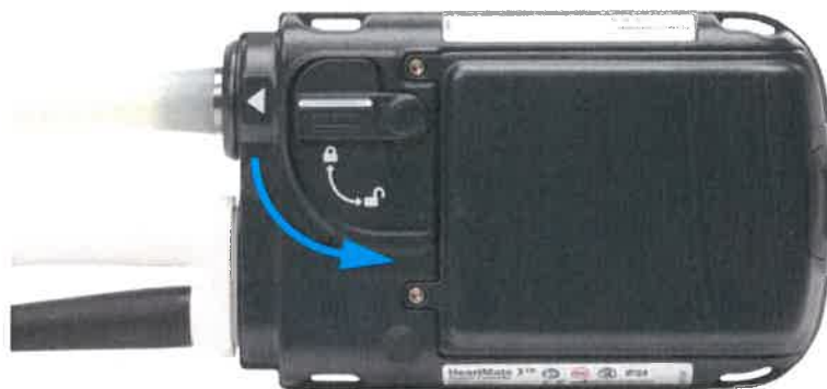
Figure 2.13 Unlock the Safety Lock
