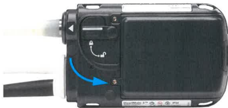
Figure 2.38 Unlock the Safety Lock
