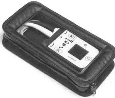
Figure 2.37 Backup System Controller in Protection Bag
