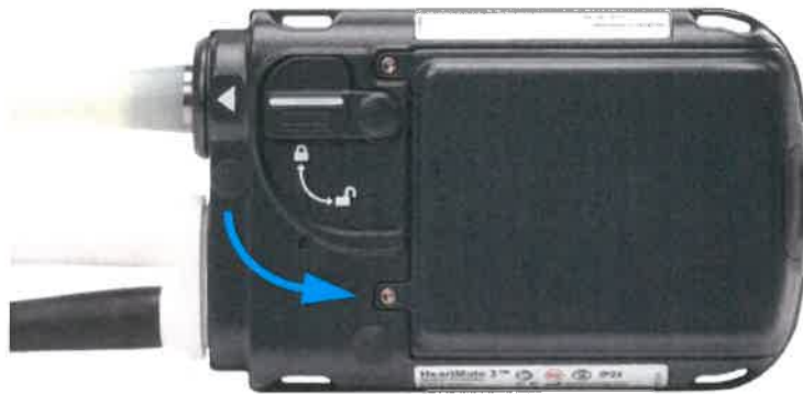
Figure 2.52 Unlock the Safety Lock
