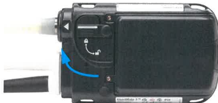
Figure 2.45 Closing the Safety Lock
