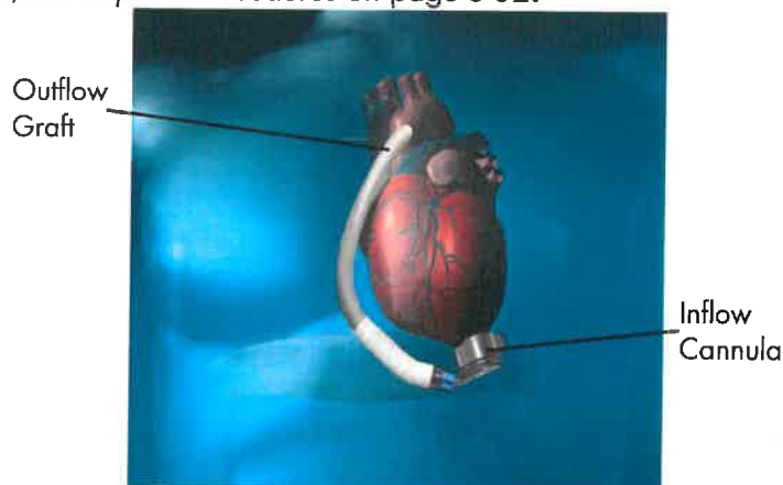
Figure 2.2 HeartMate 3 Implant Configuration
