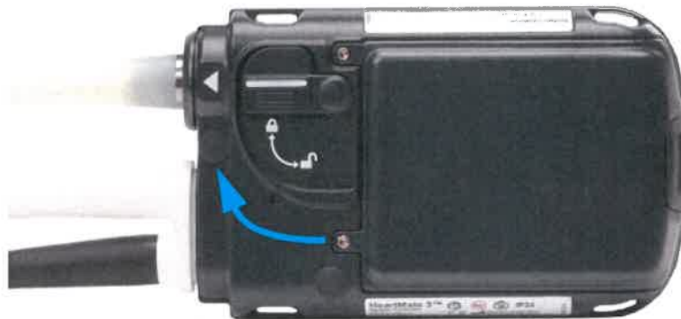
Figure 2.47 Closing the Safety Lock
