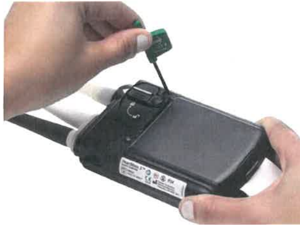
Figure 2.26 Use the Screwdriver to Loosen the Screws
