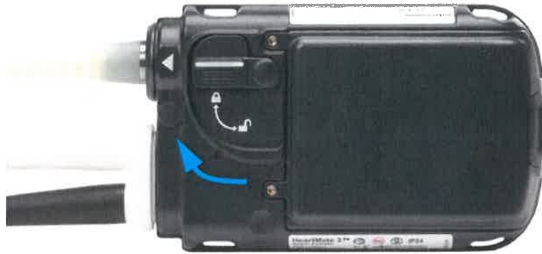
Figure 2.56 Closing the Safety Lock
