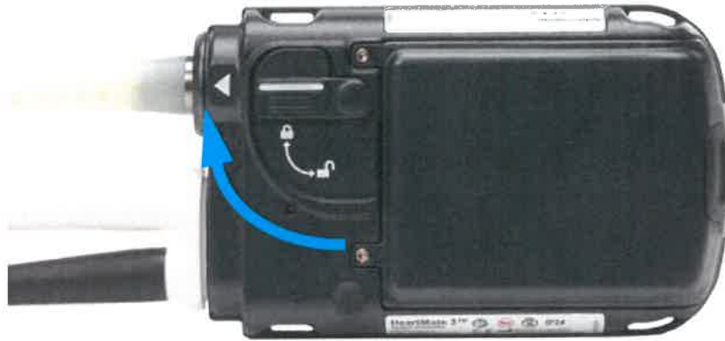
Figure 2.41 Closing the Safety Lock
