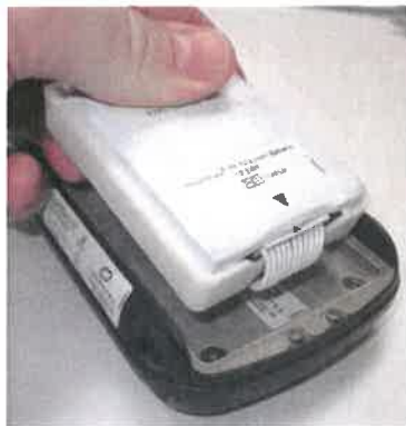
Figure 2.27 Remove Ribbon Cable from Battery Socket
