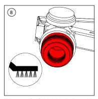
Using a small soft bristle brush, thoroughly clean the interior and exterior of the valve body, the valve body threads, the valve o-ring groove, and the valve stem seat
