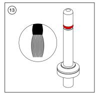
Place a very small amount of lubricant along the circumference of the valve stem's small o-ring only. DO NOT apply lubricant to the valve stem seat/gasket.
