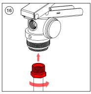
Turn siphon tube assembly clockwise into the valve body. Tighten to 5 foot pounds of torque.
