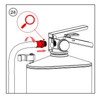
Check the hose and nozzle assembly for blockage and foreign material. Reinstall the assembly onto valve body by turning clockwise.
