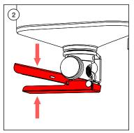
Invert the extinguisher and discharge all remaining pressurized gas.
