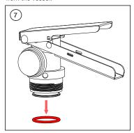
Remove the valve o-ring part no. LS-C-70060.
