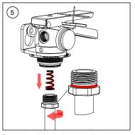
Rotate the siphon tube assembly counter clockwise to detach it from the valve body. Remove spring. Inspect siphon tube bushing o-ring part no. LS-C-60250. Remove and replace o-ring if damaged.
