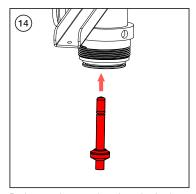
Re-insert valve stem into the valve body. Push into place with finger.
