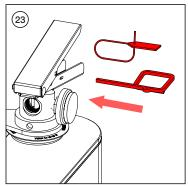
Install the pull pin part no. LS-C-60530 through upper handle / discharge lever. Attach a new tamper seal.
