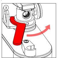
Return the extinguisher upright and set on workbench. Using Oval Brand Fire Products spanner wrench, rotate the union nut counter clockwise until the valve is free from the vessel.
