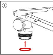
Carefully inspect the new valve o-ring part no. LS-C-70060 and install onto the valve
