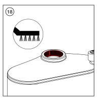
Using a small soft bristle brush, thoroughly clean the vessel's female threads, the pressure relief groove, and the o-ring sealing surface.
