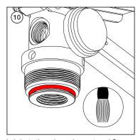
Lubricate the valve o-ring part no. LS-C-70060 along the circumference. Oval Brand Fire Products recommends Dow Corning Molykote® 55 o-ring grease.
