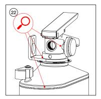
Thoroughly check all areas on the fire extinguisher that may leak; particularly welds, gauge dial and threads, valve body o-ring, and the valve stem seat.
