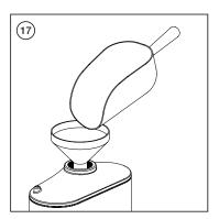
Fill the fire extinguisher vessel with the correct type and amount of dry chemical as stated on the fire extinguisher nameplate / decal.
