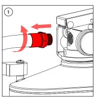
Remove the hose assembly by turning the assembly counterclockwise.
