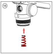
Return the spring to the siphon tube. Be careful to install it in the correct direction (larger end toward the siphon tube, smaller 8 end toward the valve stem).
