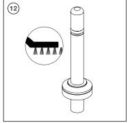
Clean the valve stem with the small, soft bristle, brush. Oval Brand Fire Products recommends replacement of the valve stem part no. LS-SS-60902 at every major service interval.
