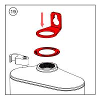
Place the mounting bracket on top of the vessel directly above the verification-of-service collar.
