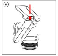
Using your finger or the pin on the spanner wrench, press down on the valve stem located under the discharge lever (upper handle).
