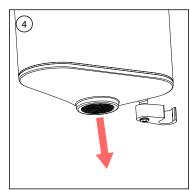
Invert the vessel to remove any remaining dry chemical powder.
