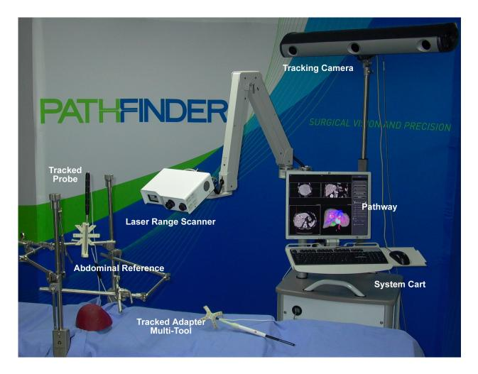
The Explorer<sup>TM</sup> system is comprised of the following elements:
