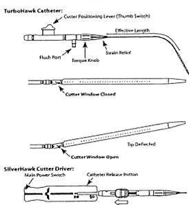
**NOTE:** The Silverhawk Cutter Driver is protected against electrical shock (double-insulated type) and against water (industrial grade IP69). The catheter is for use in the presence of a flammable anesthetic mixture. The Silverhawk Cutter Driver operates in a continuous mode and is internally powered by batteries.
