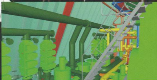
BWMS Outfitting image by 3D scanner
