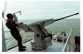
This high performance gun is designed for mounting on any type of boat or ship. Apart from its use on light patrol and combat boats, these small calibre fast-firing cannons are an ideal complement to automated weapon systems on larger vessels and play an important role in closerange defence.
