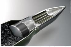
The 35mm Ahead ammunition technology consists of measurement and programming units, control electronics and programmable Ahead ammunition. It can be fitted to any suitable automatic cannon and then successfully engage small, fast aerial targets with a high kill probability. Each Ahead round contains a high number of tungsten sub-projectiles which are ejected immediately in front of the oncoming target. The measurement unit determines the velocity of each
