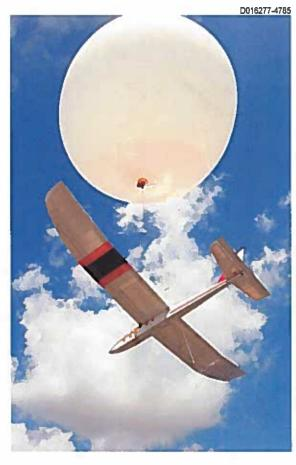
An inexpensive heliumfilled balloon launches our SkyWisp® autonomous stratospheric glider to altitudes in excess of 100,000 feet. This expendable low-cost system can carry a communications radio relay, a remoteimaging system and other payloads that require line-of-sight coverage over large areas. To date, SkyWisp has completed more than 200 successful test flights.
