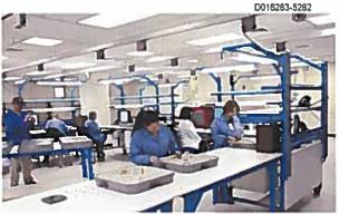
Our configurable production bay allows for fabrication and testing of a wide variety of engineering models, prototypes and hardware (pod.swri.org). Work benches, assembly and test equipment, storage cabinets and shelving, partitions, network and communication lines, and electrical power can be reconfigured quickly, as shown in these images, to meet a variety of client needs.
