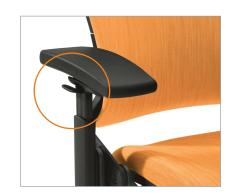
**4. Arm Height Adjustment** — Enables the user to adjust the arm height based on body size, task, and personal preference. Lift up on lever, and lift or lower arm height to desired position. Release lever to lock arm into place.
