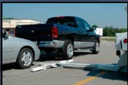
The operator extends and lowers the wheel lift to the ground while backing up to the vehicle at a 90° angle.
