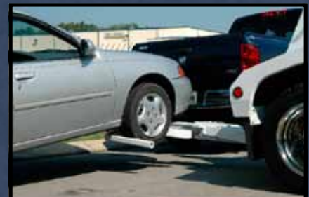
The operator now closes the arms around the tires and raises the vehicle without ever getting out of his truck. The operator is now ready to exit his truck and install the proper safety equipment.
