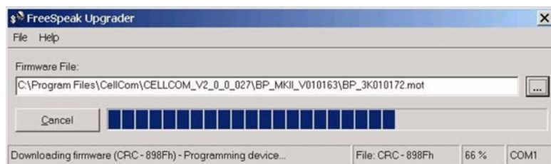
Figure 11-18: Beltpack Upgrade Progress
