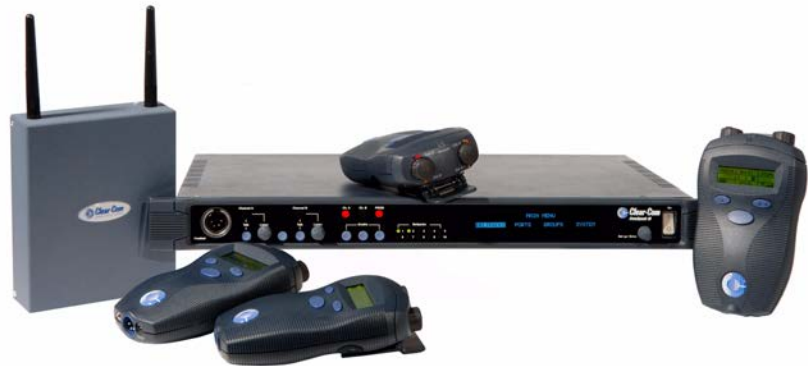
Figure 1-1: A CellCom Antenna, Beltpack, and Basestation
