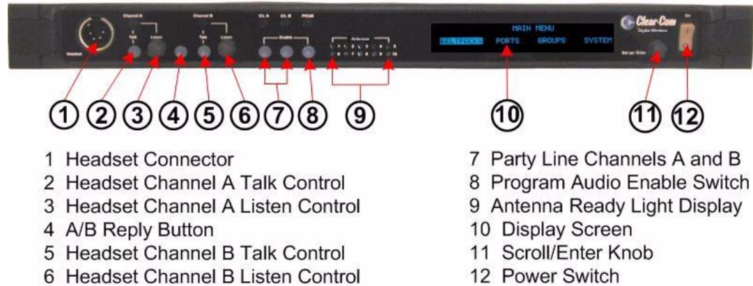
Figure 3-1: CellCom Basestation Front Panel
