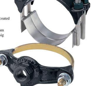
Mueller service saddles are compatible with Mueller drilling machines to install service tees. The appropriate drilling machine with equipment for the size of connection and type of pipe makes it easy to drill the main through any valve or fitting to which they can be attached. Threads in the saddles are specially designed to slightly deform the threads on the valve or fitting as it is tightened, providing a leaktight seal.
