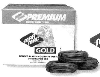
When special job specifications require the use of fusion-bonded epoxy coated rebar instead of common black steel, Mar-Mac Premium Gold offers a plastic encapsulated annealed wire that helps protect the epoxy coating and minimize corrosion. This smooth plastic coating actually bonds to the annealed wire, yet maintains the same soft, workable characteristics of all Mar-Mac Premium wire products.
