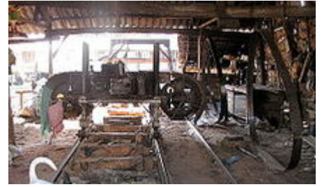
Larger resaw at a Mekong delta boatyard, fitted with a 150 mm (6") blade
