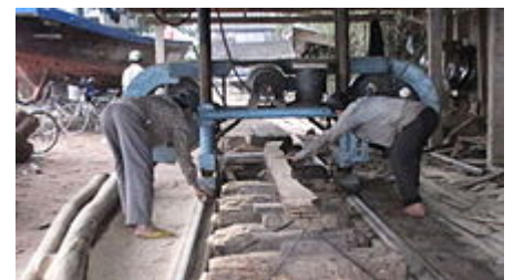
Horizontal bandsaw resawing planks at a boatyard in Hoi An, Vietnam
