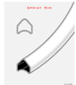
Rims for tubular tires, referred to as "sprint rims" in Britain and Ireland.
