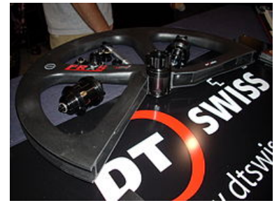
A sectioned, carbon-composite, rear wheel for mountain bikes.
