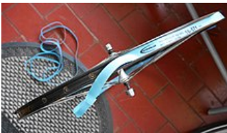
Fitting rim tape around 26 inch wheel (MTB). Rim tape protects the bicycle wheel's inner tube from spoke holes, which will puncture the tube if exposed inside the rim.
