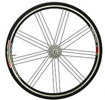
A Campagnolo rear wheel with "G3" triplet spoke lacing. There are 18 tangential spokes on the right side, but only 9 radial on the left. Picture also shows a 10-speed cassette
