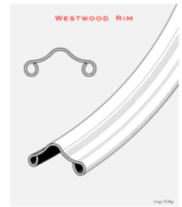
Westwood rim as fitted to vintage roadster bicycles with rod/ stirrup brakes, today being used in contemporary "drum brake" traditional utility bicycles
