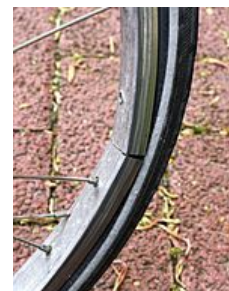
Broken rim after a bicycle/car-door collision
