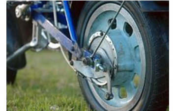
Rear wheel of 1960s Bootie Folding Cycle with Sturmey-Archer drum brake
