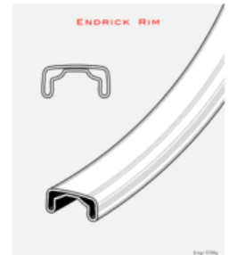
Endrick Rim as fitted to sports bicycles from the 1930s, 40s and 50s, forerunner of modern-day rim brakes
