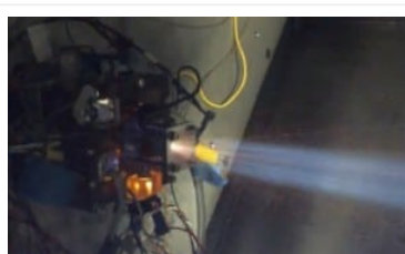
Test firing of the Hydros thruster in a vacuum chamber. Photo: TUI
