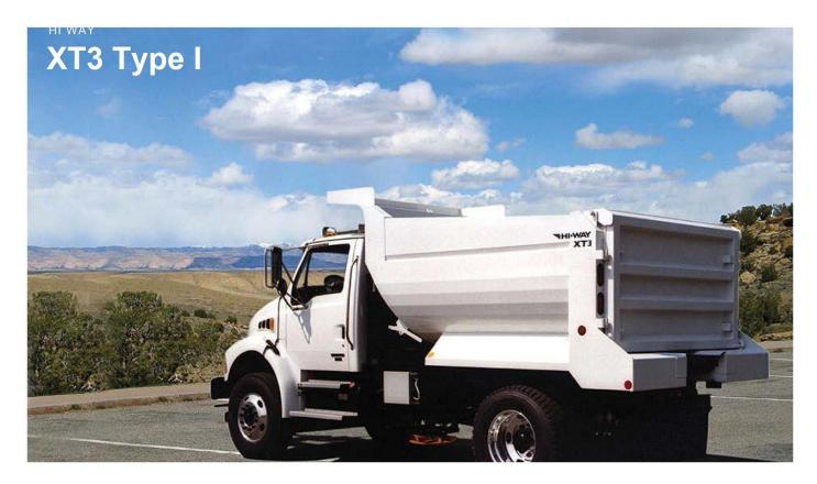
The XT3 Type I multi-purpose dump body is built for versatility. The optional front-cross conveyor give operators the ability to spread deicing material at the front or rear of the machine. They quick-detach front and/or rear spinner assemblies adjust up/down, side-to-side, and fore/aft for a consistent spread pattern, and the flat dump body floor lets operators haul virtually any material.
