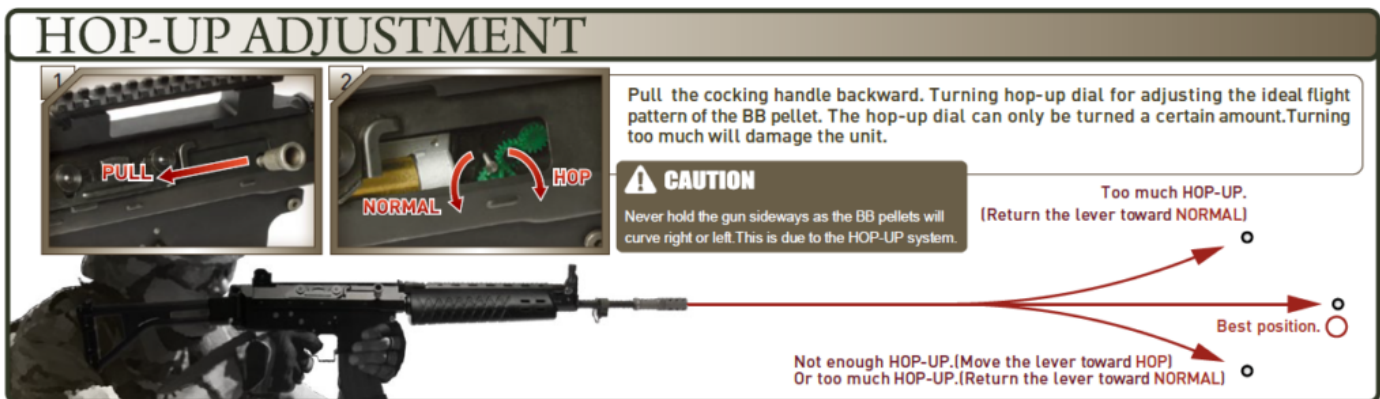
The effect of hop-up adjustment.
