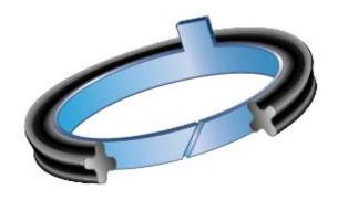
A tab on the thermoplastic ring locks it into the housing or shaft to prevent independent movement of the seal assembly. The ring is split to allow for thermal expansion of the shaft or cylinder.
