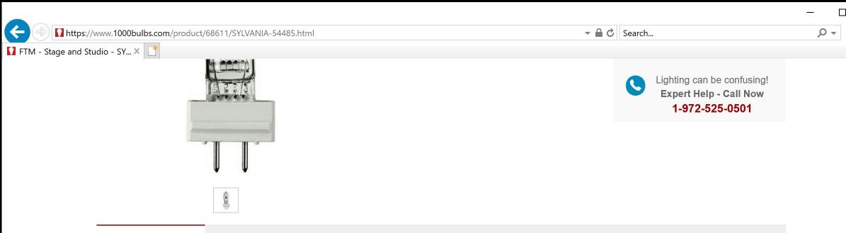
**Brand** SYLVANIA MPN (Part No.) 54485 GY16 Base Type T34 **Bulb Shape Burn Position** Base Down +/- 90 Degrees **ANSI Code** FTM Life Hours 400 Wattage 2,000 Watt
