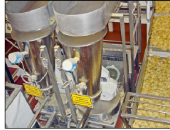
Coperton K-Tron feeders in a snack food process
