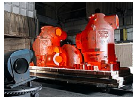
Steel castings after undergoing 12-hour 1,200 °C (2,190 °F) heat treatment.
