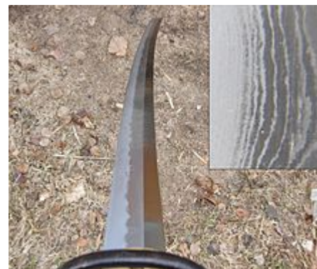
A differentially hardened katana. The bright, wavy line following the hamon, called the nioi, separates the martensitic edge from the pearlitic back. The inset shows a close-up of the nioi, which is made up of individual martensite grains (niye) surrounded by pearlite. The wood-grain appearance comes from layers of different composition.
