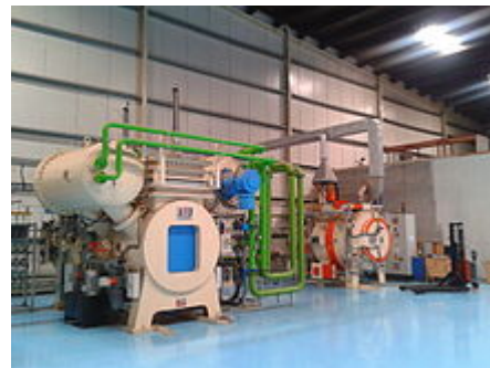
A modern, fully computerised case hardening furnace.
