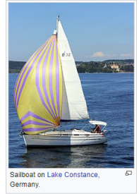
A typical monohull sloop with Bermuda rig
