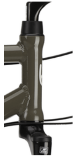
Threaded headset with internal bearings on 2016 Brodie Quantum bicycle
