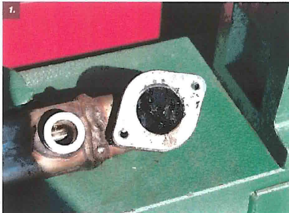
1. On 6.0L Power Strokes, the question is not if the EGR cooler is going to fail, but when. Take a look at the gunk buildup inside this EGR cooler. Not much flow going on here.
