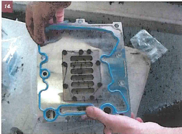
14. The bottom of the manifold features a much larger opening and filter screen than the stock unit for feeding the high-pressure oil pump. Aircraft safety wiring makes sure the bolts won't back out and drop into the engine.
