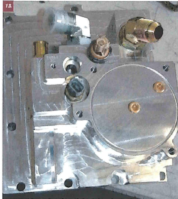
13. The heart of the Bullet Proof Diesel engine-oil cooler kit is this billet manifold that sits on top of the engine in place of the factory oil manifold. It has AN fittings for both input and output lines, and provisions for the factory sensors.
