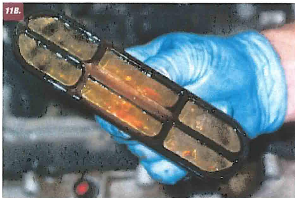
11A & B. Another problem area is this screen setup that sits under the oil cooler. The screen filters oil that flows into the high-pressure oil pump that operates the 6.0L fuel injectors. Over time, the screen gets plugged with debris (seen here) or starts to deteriorate on its own, according to Bullet Proof Diesel.
