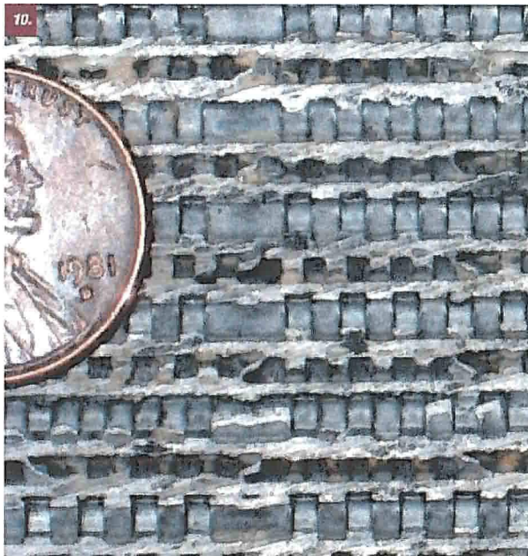
10. A cutaway of the factory cooler shows how tiny the factory oil and coolant passages are. Bullet Proof Diesel asserts when these coolant passages plug up with debris, it leads to EGR failures and eventual failure of the oil cooler, not to mention bigger problems down the road.
