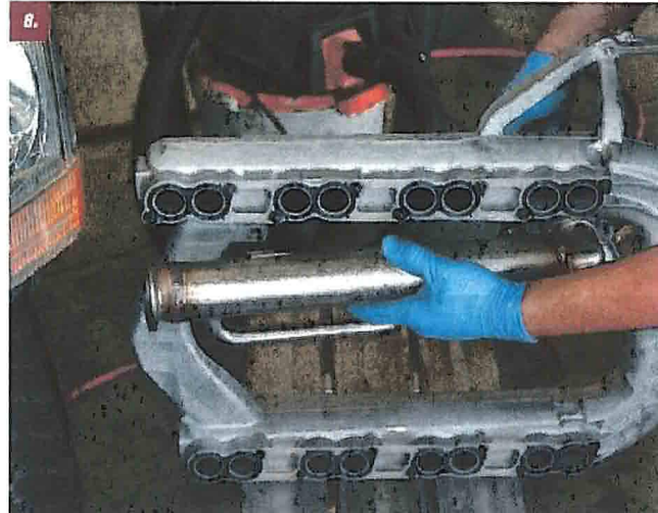
8. The EGR cooler is mounted to the bottom of the intake manifold and returns coolant through passages in the manifold.
