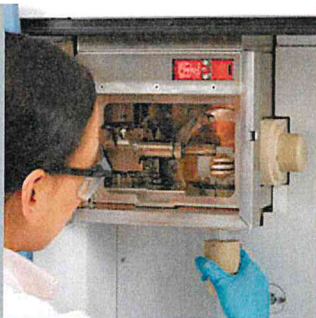
1) Simply remove radial torch and interface
