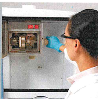
3) Install axial torch and interface
