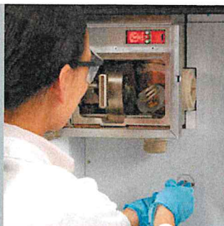
2) Rotate load coil into desired horizontal orientation
