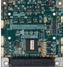
ADCS Board – developed from our experience with the DICE and DIME CubeSat missions, this 2-axis spin-stabilized control provides an affordable yet robust solution for meeting CubeSat pointing requirements.
