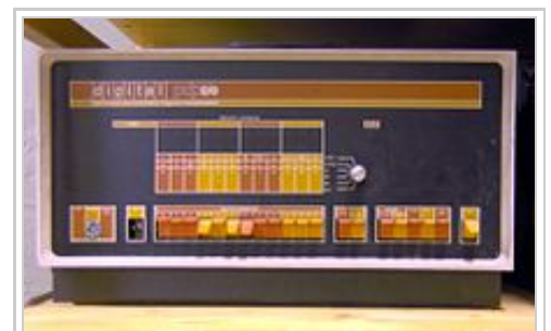
PDP-8/E front panel showing the switches used to load the bootstrap program
