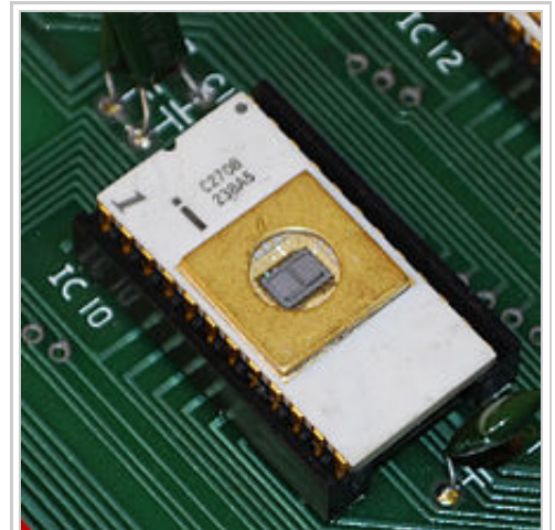
An Intel 2708 EPROM "chip" on a circuit board.
