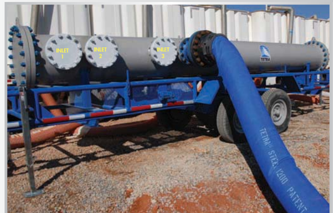
Ability to Blend Process Water from Multiple Sources Blended in a Patent-Pending Manifold
