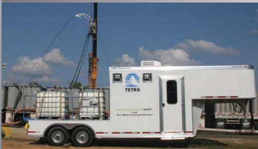
Mobile Unit for On-The-Fly Water Treatment and Recycle and Reuse of Process Waters
