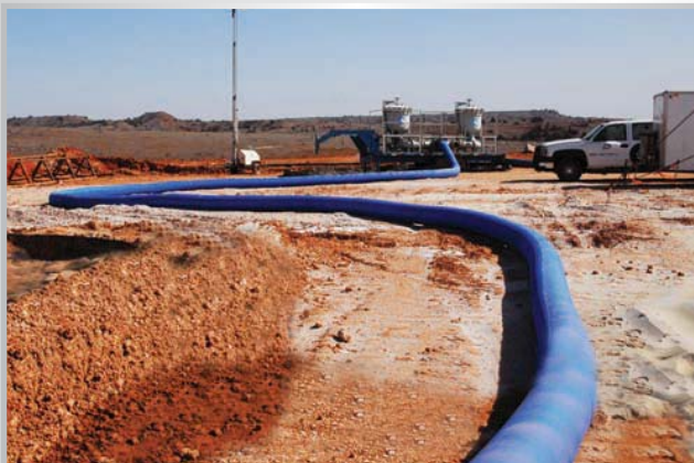
500’ Lengths; 11 Connections per Mile; 200 BPM, Single-Line Capacity, Flexible Conduit; Less Connections vs Conventional Jointed Pipe
