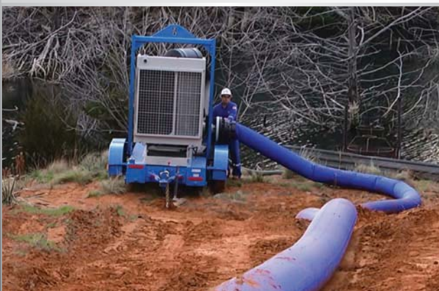
575 HP, High Rate, High Pressure Pump Unit Maximizes TETRA® STEEL 1200 200 psi Working Pressure with 3X Safety Factor
