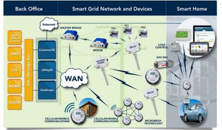
An advanced, IP-based network enables the smart grid—from the data center to the customer premise.
