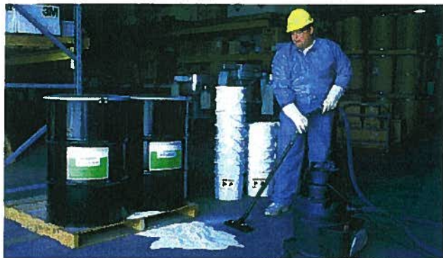
Recommended personal protective equipment includes gloves, safety glasses or goggles, and long sleeves.
