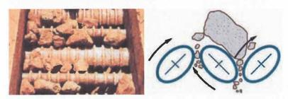
Our wobbler feeders operate with low horsepower and headroom requirems without vibration, noise or transmitted stresses, making them ideal for both and portable applications.
