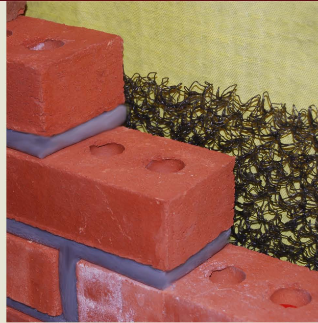
The entangled matrix design of the Blockade™ Mortar Deflection System traps mortar droppings and allows excess moisture to flow freely out of the wall cavity.
