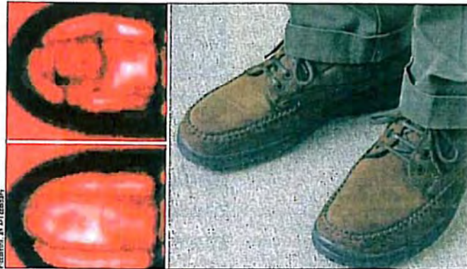
Threat detection: THz imaging can be used to locate and identify explosives (present here in the top scan).
