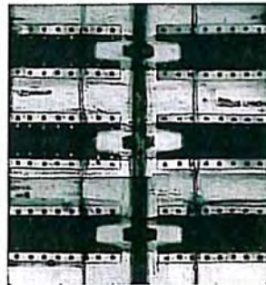
FIGURE 5. Terahertz images of foam insulation (light areas) on the external fuel tank of the space shuttle. Voids within and delamination between layers of foam insulation appear as dark areas. This composite image shows 25 defects, only two of which are visible on the exterior of the foam.
