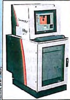
Picometrix's commercially available QA1000 THz imager forms part of the high-speed scanning set-up.
