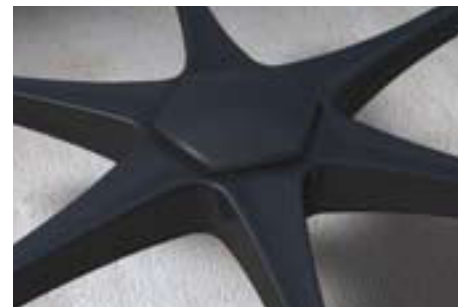
Node structure providing junction efficiency of 100%.
