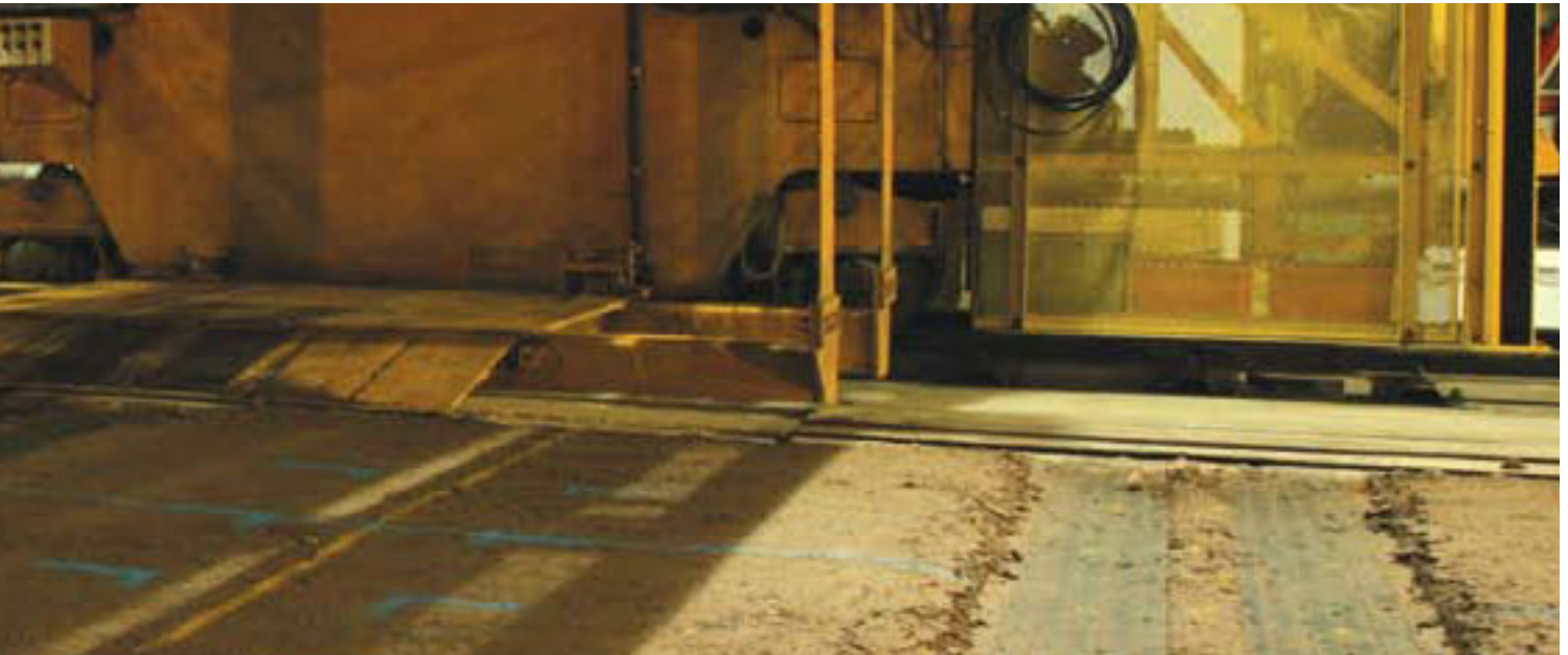
Trafficking trials at TRL proved the performance benefits of the TriAx geogrid compared with biaxial geogrids.
