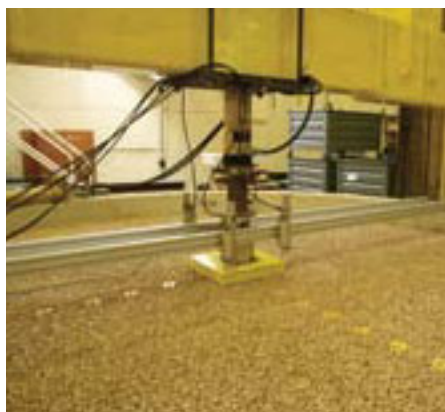
Bearing capacity tests at BRE confirm TriAx geogrids increase load distribution.
