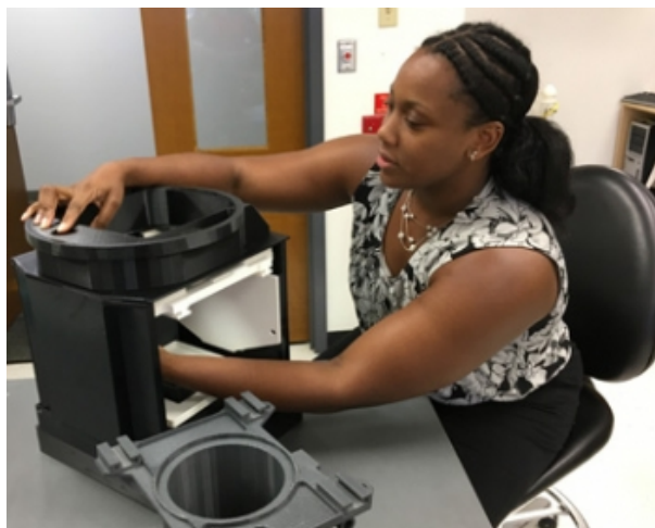
An Aerospace intern works on a 3D-printed NIRAC model she designed to help assembly technicians determine how to route internal NIRAC cables. (Photo: Laura Johnson/Aerospace)
