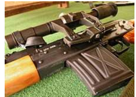
Romanian PSL rifle with Warsaw Rail a variation of a dovetail used for scopes from 1954. Becoming common on the AK-### series as of 1992
