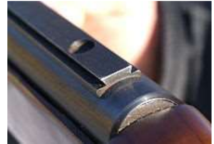
A dovetail rail on a rifle receiver for mounting a sight (i.e. a scope or iron sights).
