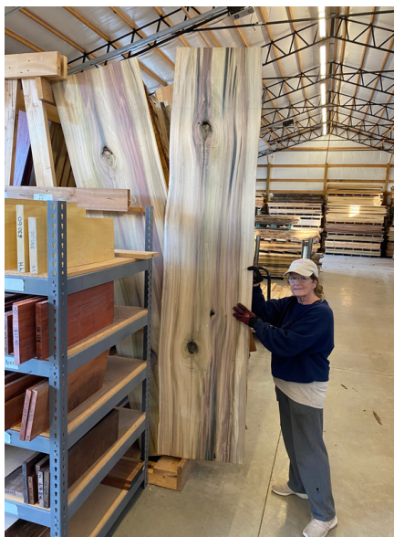
Big, 2 inch thick live edge slabs
