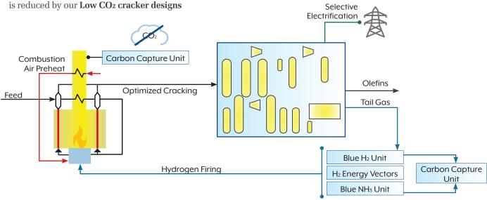
KBR is developing concepts for steam cracking furnace electrification, for not to completely removing the flue stacks and direct emissions from pyrolysis furnaces.
