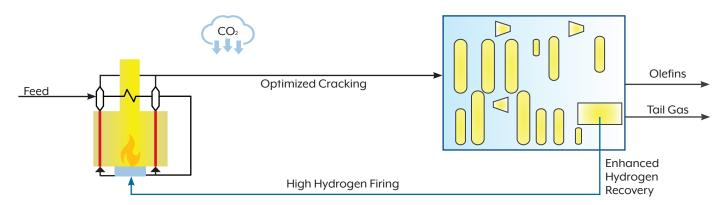
KBR SCOREKlean services provides Low CO2 cracker design, emission reductions without requiring carbon capture or an external source of hydrogen. Our emission reduction designs remove carbon from the pyrolysis furnace firebox and move heat from the steam system into the process.
